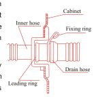
It had better put the outlet of the drain hose into the nearby drainage permanently, which can save the trouble that the drain hose has to be connected each time before use. If the drainage is far from the washing machine, it can be solved by connection of the drain hoses head with end to extend.
